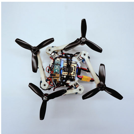
When faced with a narrow passage, the drone can switch to a "O" shape, with all arms folded as close as possible to the body. (Image: UZH)
