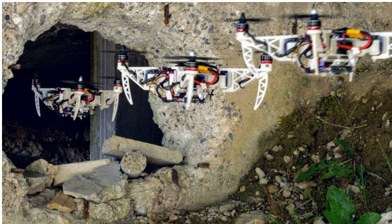
The morphing drone can squeeze itself to pass through gaps and then go back to its previous shape, all the while continuing to fly. (Image: UZH)
